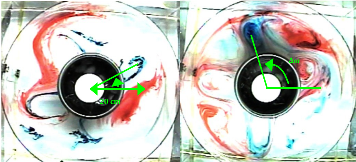
Figure 5. Speed estimation for eddies. Each eddy has an angular velocity, estimated by the green line segments. Multiplying the angular speed by 20 cm yields an estimate of the eddy linear speed.
