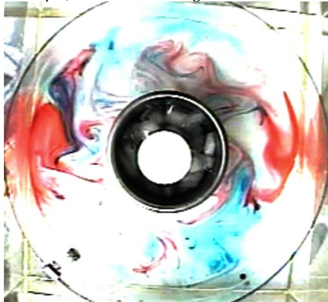
Figure 3. Eddies observed for the fast rotation (10 rpm) case.
