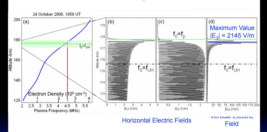
Large Increase in Electric Field Just Below Reflection Altitude where EM Wave Frequency = Plasma Frequency
