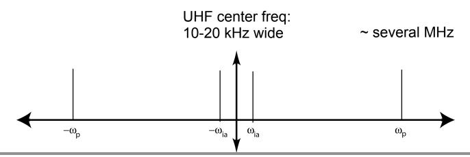
Why aren't the Langmuir (plasma) waves damped? Electron thermal velocity ~ 125 km/s but plasma wave frequency ~ several MHz – Not much interaction and not much damping.
