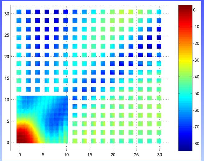
Comparison of the geometric distance between the cal antenna and individual AEUs with the NEC computed phases shows the effects of the antenna phase functions and scattering. Note that in this case the errors are systematic and have magnitudes as large as ~90 degrees. Other geometries can result in even more dramatic effects.
