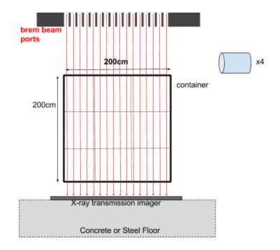
3) Where would the smuggler locate the WGP? Where would you (i.e. the inspector) put your four neutron detectors, to maximize the neutron signal (while keeping in mind that the smugglers know the system configuration)? Re-draw this on the board and mark it up. Would you rather have the floor made of concrete or steel, and why?
