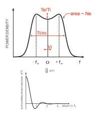
Ion temperature (Ti) to ion mass (mi) ratio from the width of the spectra
