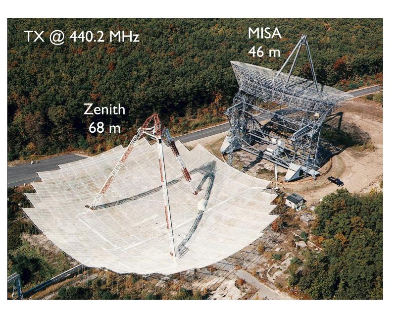
This is an experiment designed to observe rapid oscillations in the mid-latitude ionosphere generated from traveling ionospheric disturbances (TIDs), the passage of the solar terminator, and other related effects. Alternating observations are used between the zenith and MISA antenna pointing up the local magnetic field line at 250 km altitude.
