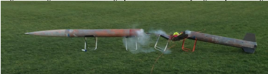
Figure 19 - Image of the drogue being drawn out of the rocket tube - a sign of a successful ejection event
