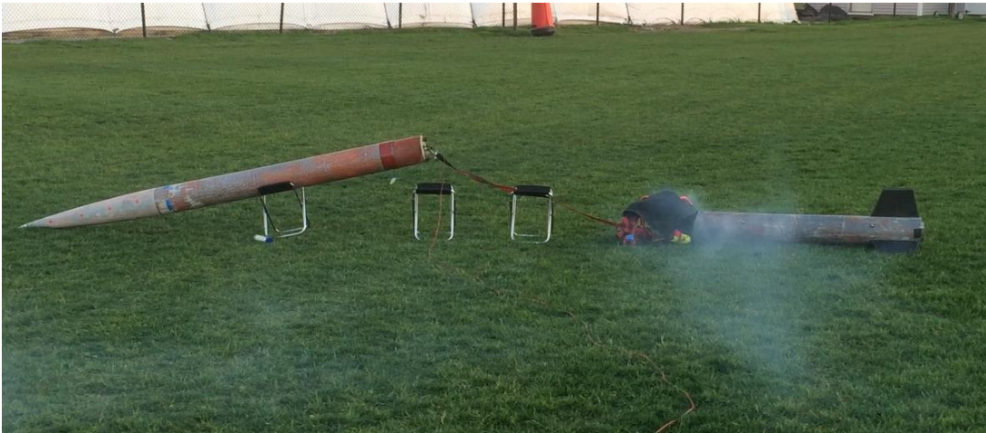
Figure 18 - Image of the rocket following separation of the fin can by a 3g black powder charge
