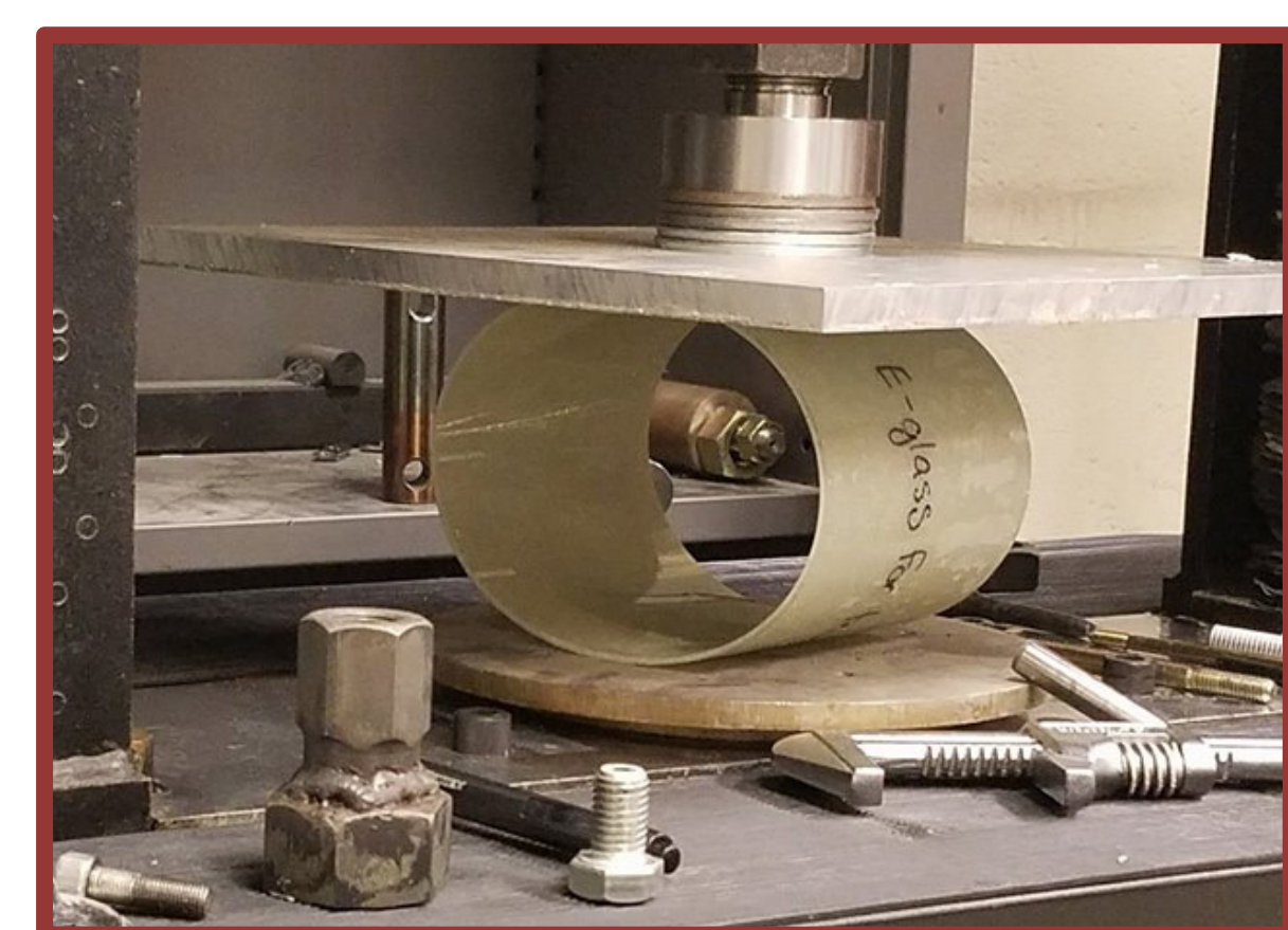
Fig 7: Crush testing tubes
