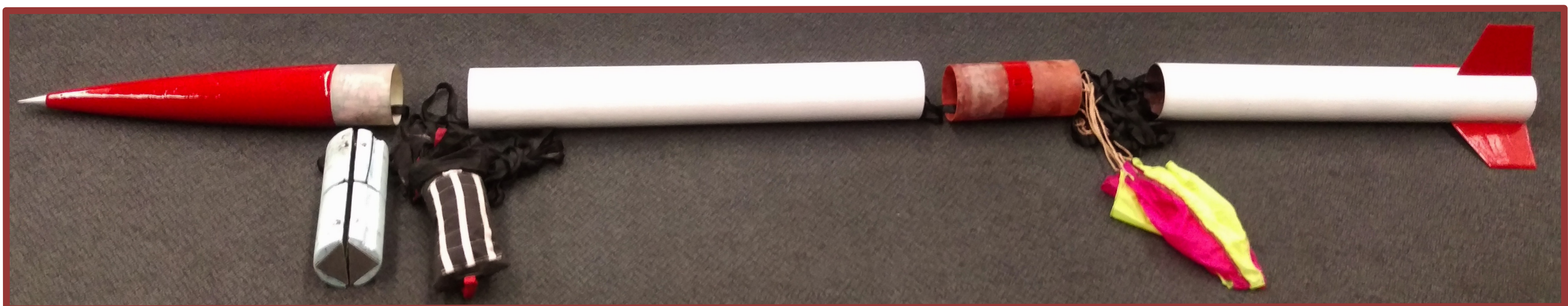
Fig 10 (bottom): Laying out the different sections of the rocket along with all recovery components during the final assembly process before IREC.
