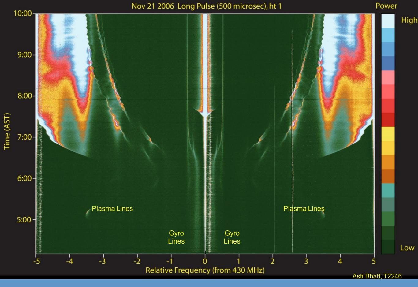
Arecibo Sensitivity: The 305 m dish, 2.5 MW of power, and Tsys of about 80 K (condition dependent) provide high time resolution on even weak features such as the gyro line. The data above are centered on the E region. The strong plasma line after sunrise is "leakage" from the low F region. The complicated behavior of the gyro line is probably due to multiple layers, but is not completely understood.!
