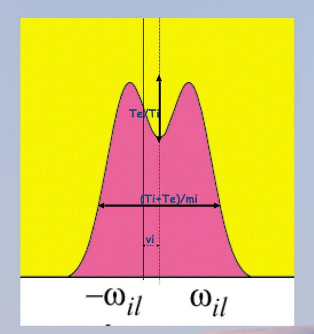
•Ion (and electron) temperature (Ti and Te) to ion mass (mi) ratio from the width of the spectra
