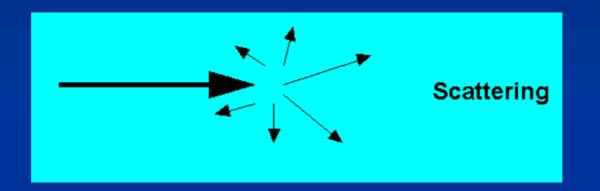
• In the low-energy limit, the electric field of the incident wave (radar wave) accelerates the charged particle, causing it, in turn, to emit radiation at the same frequency as the incident wave, and thus the wave is scattered.
