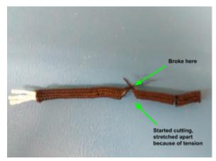
The ropes tended to break in a distinct triangle pattern. The current required was about 2.3 amps (3.4 volts) for about 10 seconds before it broke.
