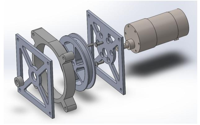
Manufacturing: mostly waterjetting, a little bit of countersinking, tapping, turning. Weight as of now: 0.8029 (1 motor and 1 drum).
