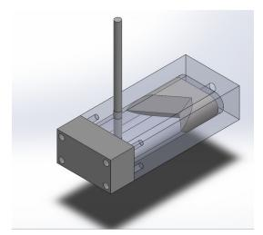
need to figure out manufacturing, not sure we will be able to make the slot that the knife slides along. Also need to do research on how tight the tolerance needs to be between the knife, pretty much concerned about the gas escaping around the knife. need to figure out a way to quantify that shit as well as determine what the cutting force is going to be. Thinking it might be fun to just test that shit.
