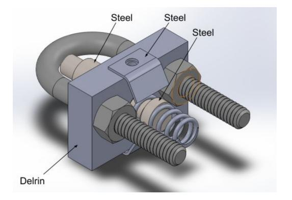
The <u>spring</u> exerts 26lbs of force. The minimum gauge of wire that will support this is 22AWG nichrome wire. So, for safety, use 18AWG wire.
