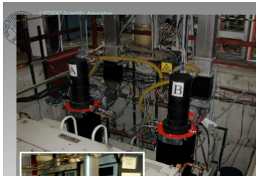
A 60-kW VHF klystron (500 MHz) at ESR.
