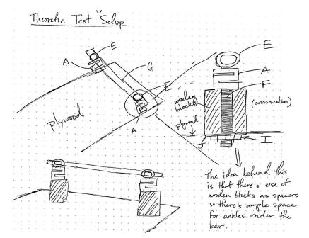
(Key: **A** - Load Cell, **E** - M12 Eye Ring Bolt, **F** - M12 Threaded Rod, **G** - 1" Aluminum Rod, **I** - M12 Hex Nut, **J** - M12 Washers)
