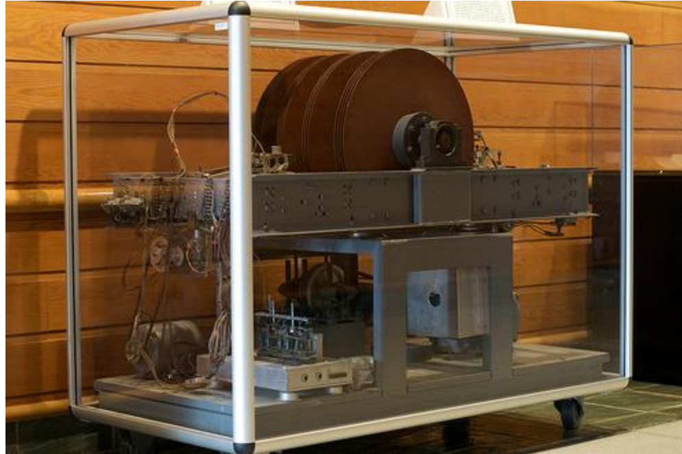
The world's first hard drive, IBM Almaden Research Center in 1952-1954 (5Mb)
