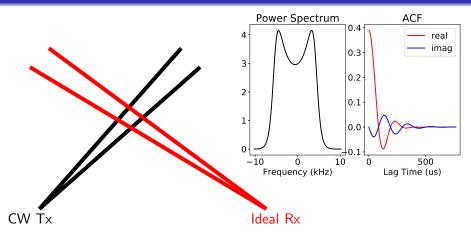
ISR theory gives the PSD and ACF of the received voltages as a function of  $N_e$ ,  $T_e$ ,  $T_i$ , and  $u_{los}$  in the overlap volume.
