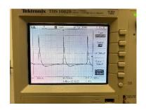
Pulse Energy = 387 nJ @ 50 Hz BW set to 150 Hz
