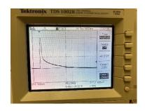
Pulse Energy = 387 nJ @ 10 Hz BW set to 150 kHz
