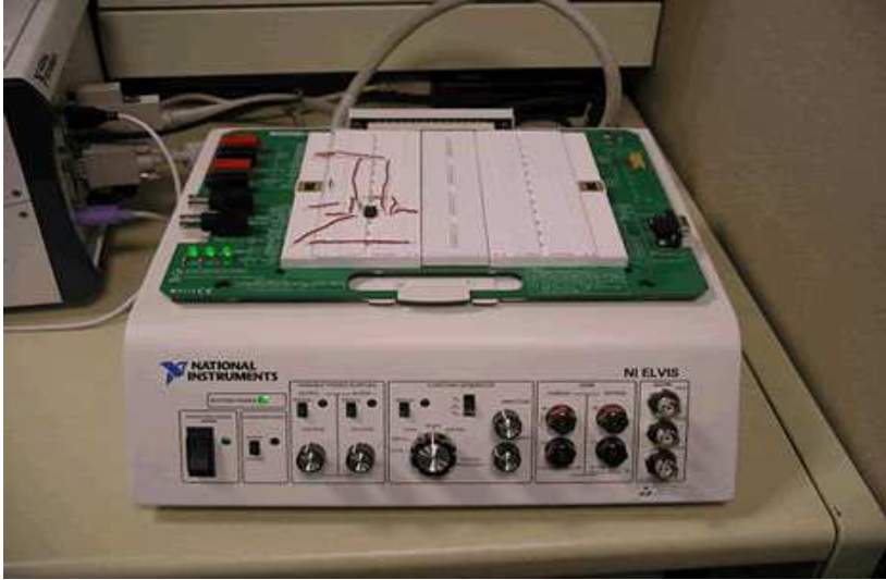
Figure 2-2: This is a diagram of the ELVIS workstation with a simple circuit constructed on its prototyping board. The knobs on the front can be used to control the workstation manually.
