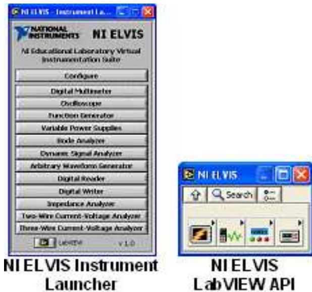
Figure 2-3: The ELVIS instrument launcher gives users access to LabVIEW built virtual instruments that can control the ELVIS workstation. The source code for these instruments is provided and can be added to LabVIEW virtual instruments.
