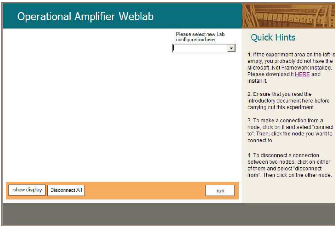
Figure 3-6: This page of the OAU opLab client presents the user with a choice of operational amplifier configurations.
