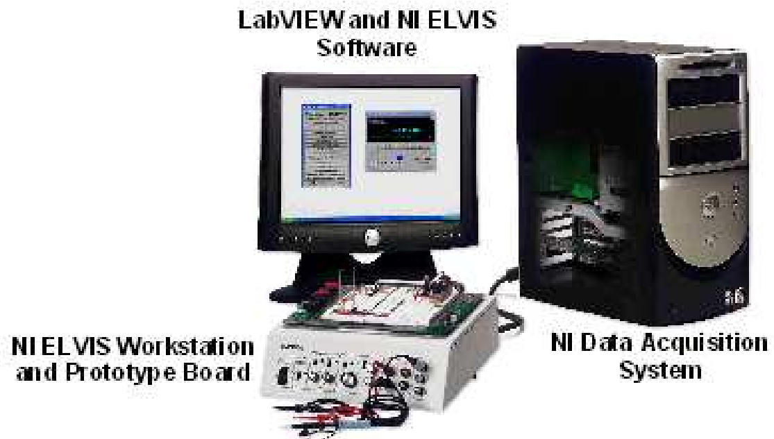
Figure 2-1: This diagram shows the three components that make up the ELVIS platform.
