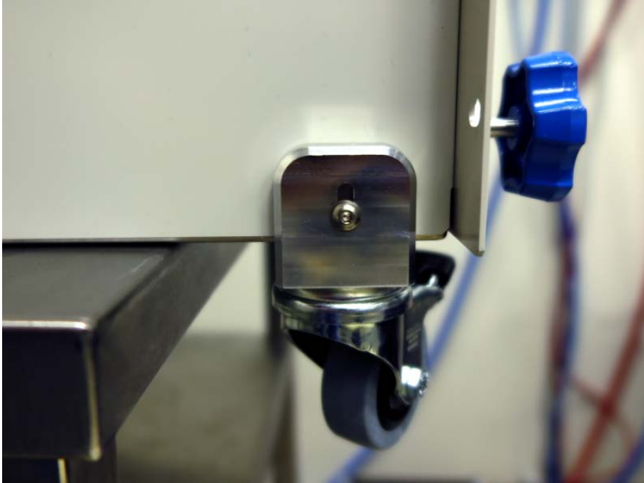
Figure 33. SMC Chiller - view of the attached wheel to the chassis
