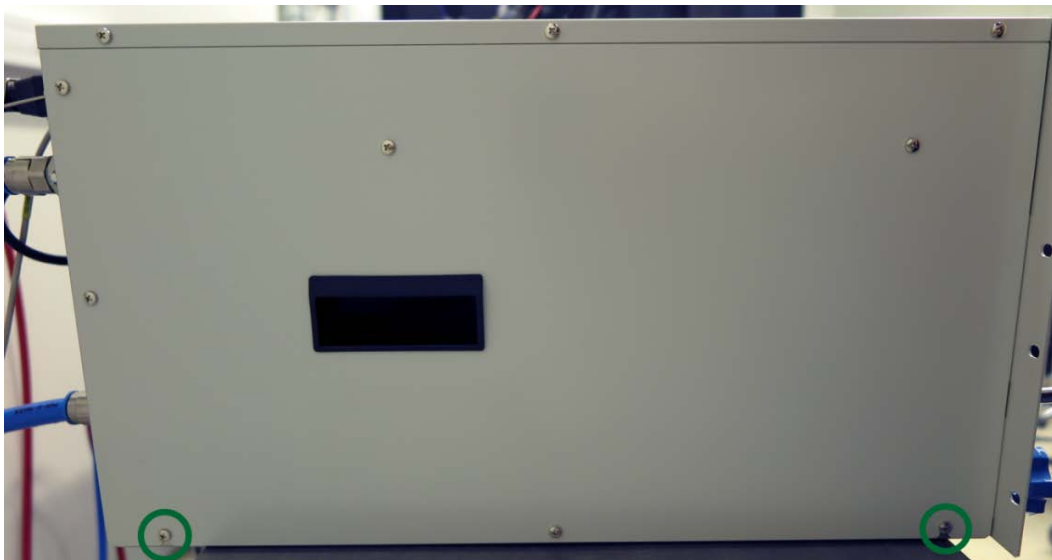
Figure 32. SMC Chiller chassis fixation holes for the attachable legs modification
