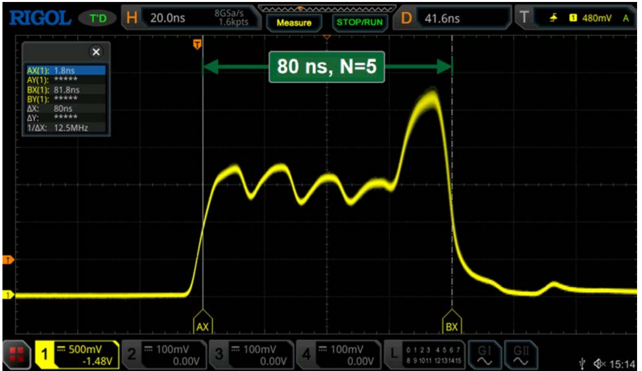
Figure 46. Display of the adjusted nanosecond pulse on the oscilloscope (N=5)
