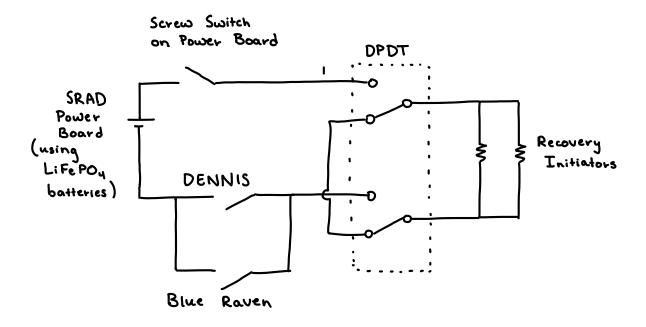
· Note: Both DENNIS and Blue Raven used for recovery initiation redundancy (ensures 2 independently powered COTS computers firing recovery, not only the Telemega)
