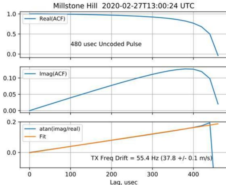
Radar data is obtained using real hardware and requires calibration:
