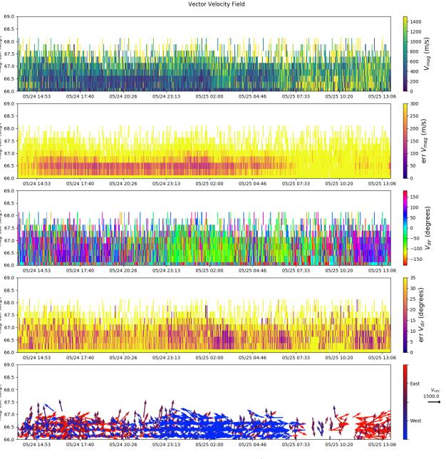
You can get resolved vector velocities/electric field from any experiment with 3 or more beam positions
