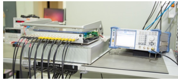
Lower: FSRU testbench used during serial production
