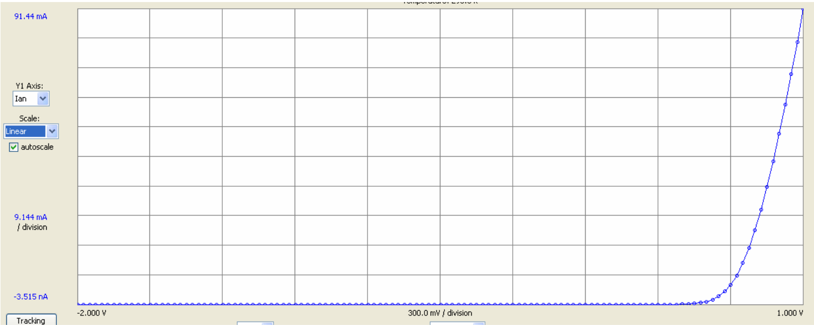
Graph 1: Linear plot of the diode current versus applied bias
