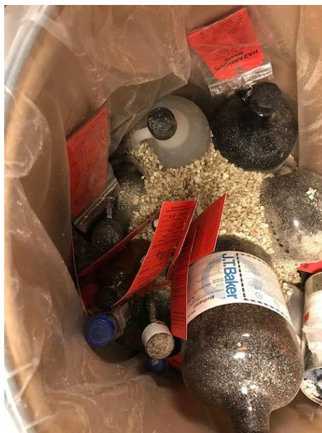
Figure 25: Photo of lab-packed bottles. Photo source: MIT EHS.
