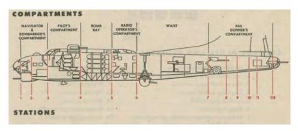
Figure 4.13 The crew compartment layout in the B-17<sup>87</sup>
