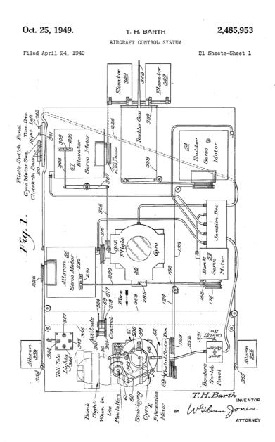
Figure 3.15 The SBAE as shown in "Aircraft Control System" Patent No. 2,485,953, filed by Theodore Barth.<sup>116</sup>
