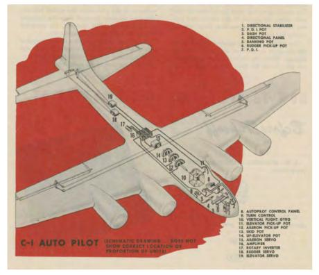
**Figure 3.20 B-17 C-1 Autopilot schematic drawing**<sup>155</sup>
