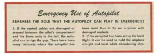
**Figure 3.19 Emergency Use of Autopilot entry in the** *B-17 Pilot Training Manual*<sup>151</sup>
