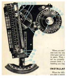
**Figure 4.18 The Automatic Bombing Computer**<sup>102</sup>
