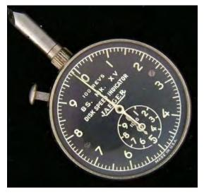
**Figure 5.41** Norden bombsight Jaeger tachometer<sup>154</sup>
