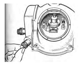
**Figure 5.15** The vertical gyroscope leveling knobs<sup>49</sup>
