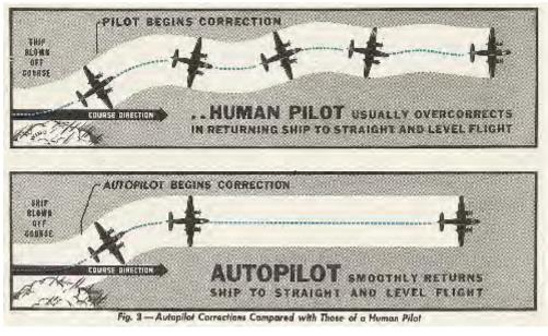
**Figure 3.21 Precision flying and the pilot vs. the autopilot**<sup>157</sup>
