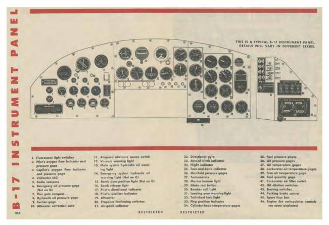
Figure 3.10 B-17 Pilot Cockpit Instrument Panel<sup>94</sup>
