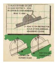
**Figure 4.6** Weems plotter and course measurement<sup>59</sup>
