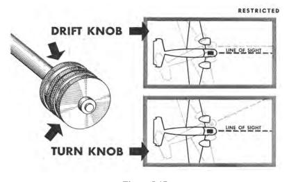
**Figure 5.17 The drift and turn knobs**<sup>54</sup>
