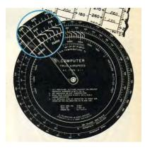
Figure 5.30 G-1 True Airspeed Computer<sup>122</sup>
