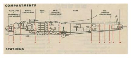
Figure 2.2 The B-17 crew compartment layout<sup>78</sup>
