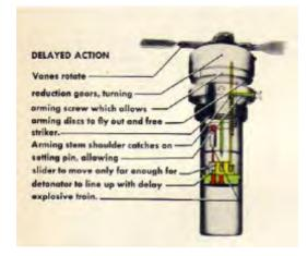
Figure 5.38 AN-M103 Delayed Action Arming Vane Nose Fuze<sup>142</sup>
