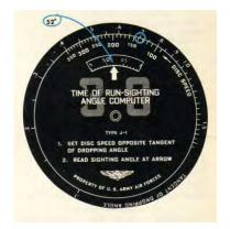
**Figure 5.31** J-1 Time of Run-Sighting Angle Computer<sup>123</sup>
