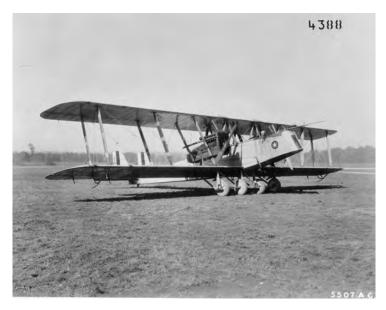
Figure 3.3 The Glenn Martin GMB bomber, the first U.S.-designed bomber procured in quantity by the U.S. Army during World War 1<sup>46</sup>
