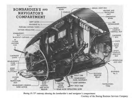
Figure 4.14 The B-17F bombardier and navigator's compartment<sup>90</sup>
