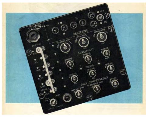
**Figure 3.23 The pilot's autopilot control panel**<sup>161</sup>
