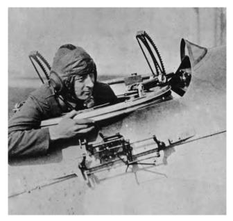
Figure 5.8 Early, non-drift setting Wimperis bombsight installed on an American DH-4<sup>22</sup>
