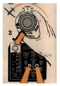
**Figure 3.25 The C-1 Autopilot Turn Control Knob**<sup>166</sup>
