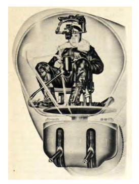
**Figure 5.37** The optical gunsight and chin turret on the B-17G<sup>137</sup>
