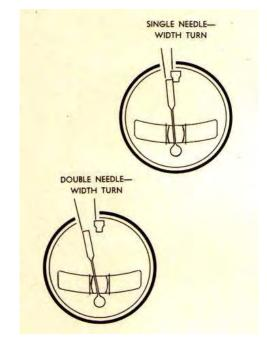
**Figure 3.11 Turn and bank indicator**<sup>105</sup>
