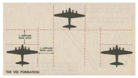
**Figure 3.6 Three aircraft element formation**<sup>86</sup>
