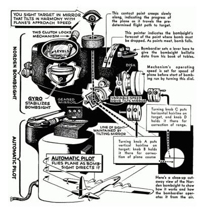
Figure 5.18 The Norden M-Series bombsight in operation<sup>59</sup>
