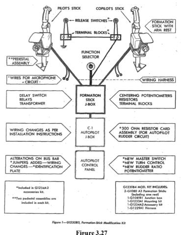
C-1 Autopilot Formation Stick system schematic diagram<sup>173</sup>
