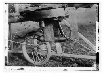
Figure 5.1 A single bomb suspended from Riley Scott's "bomb dropper"<sup>6</sup>
