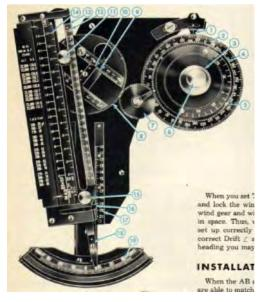
**Figure 5.32 The Automatic Bombing (AB) Computer**<sup>125</sup>
