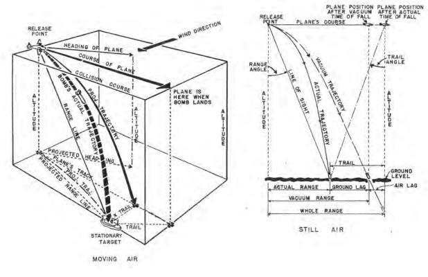
**Figure 5.6 The bombing solution**<sup>19</sup>
