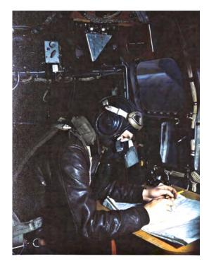
Figure 4.3 The Navigator at his workstation. Note the map, the dividers in his right hand, and the bag containing his E6-B computer to his left.<sup>33</sup>
