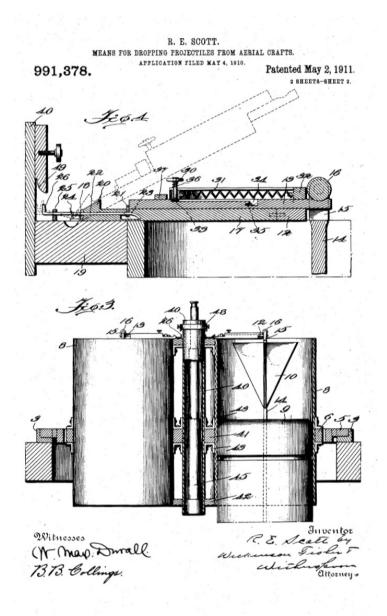
Figure 5.2 Riley Scott's "bomb dropper" device, as represented in U.S. Patent No. 991,379<sup>9</sup>
