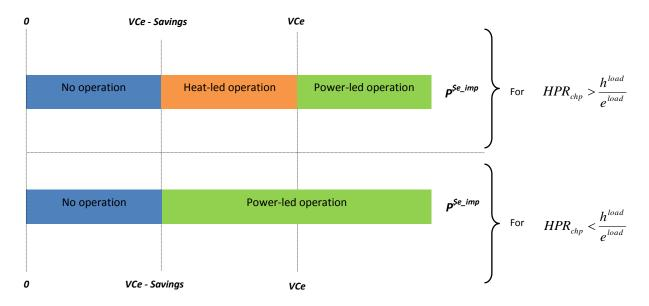
Figure 6.2.25: Micro-CHP operational outputs under different prices & load conditions
