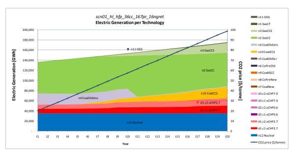
Figure 6.1.2: LT results for the case with micro-CHP - Electric generation [GWh/yr] for every year of the time horizon for conventional generating and micro-CHP technologies
