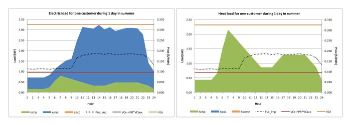
Figure 6.2.26: Micro-CHP operation with HPR2.7 for one customer, 1 day in summer under hourly (HR) rate
