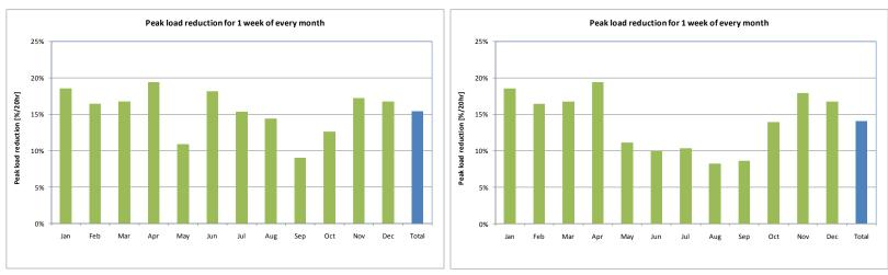
Figure 6.2.11: System's electric peak load reduction - CHP case & CHP w/o NC&GCP case vs. AFO case
