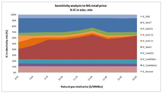
Figure 6.1.11: Percentage of electric installed capacity (IC) within the electric portfolio at the end of the time horizon, per conventional generating and micro-CHP technology (case with High CO2 price/High micro-CHP capital cost).
