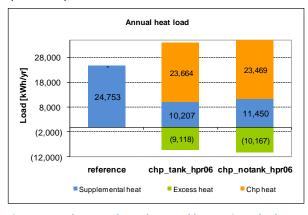
Figure 4.1.17b: Annual supplemental heat, micro-chp heat and excess heat for low HPR case
