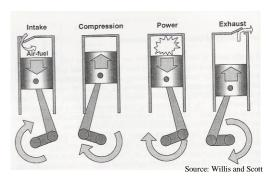
Figure 2.2.1: Otto cycle used in internal combustion engines
