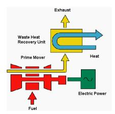
Figure 2.1.2: CHP basic operation
