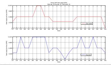
Figure 4.1.5a: One day of operation in January/Winter See oscillating operation of micro-CHP with buffer tank (blue line)
