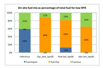
3.2-14 a considerable percentage of heat is supplied by auxiliary heating equipments. Regarding net power we note that under the least-cost strategy, the micro-CHP operates at full capacity almost the entire time as there is an incentive to export electricity back to the grid.
