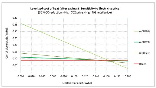
Figure 6.1.18: Heat cost considering electricity savings – Sensitivity to electricity price
