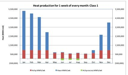
Figure 6.2.15: Total energy load supplied by conventional and micro-CHP technologies for Customers Class C1
