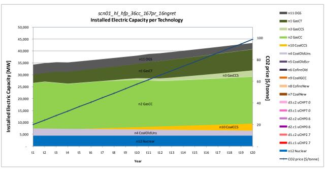
Figure C. 25 Results for the case with No micro-CHP - Electric installed capacity at every year of the time horizon for conventional generating and micro-CHP technologies
