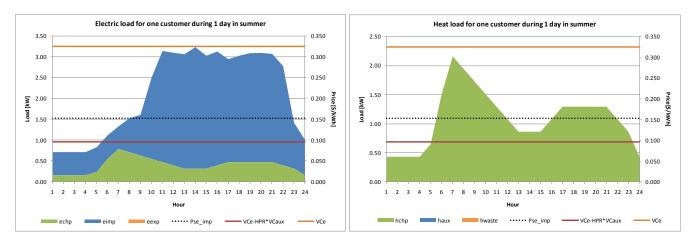
Figure 6.2.27: Micro-CHP operation with HPR2.7 for one customer, 1 day in summer under flat (FL) rate
