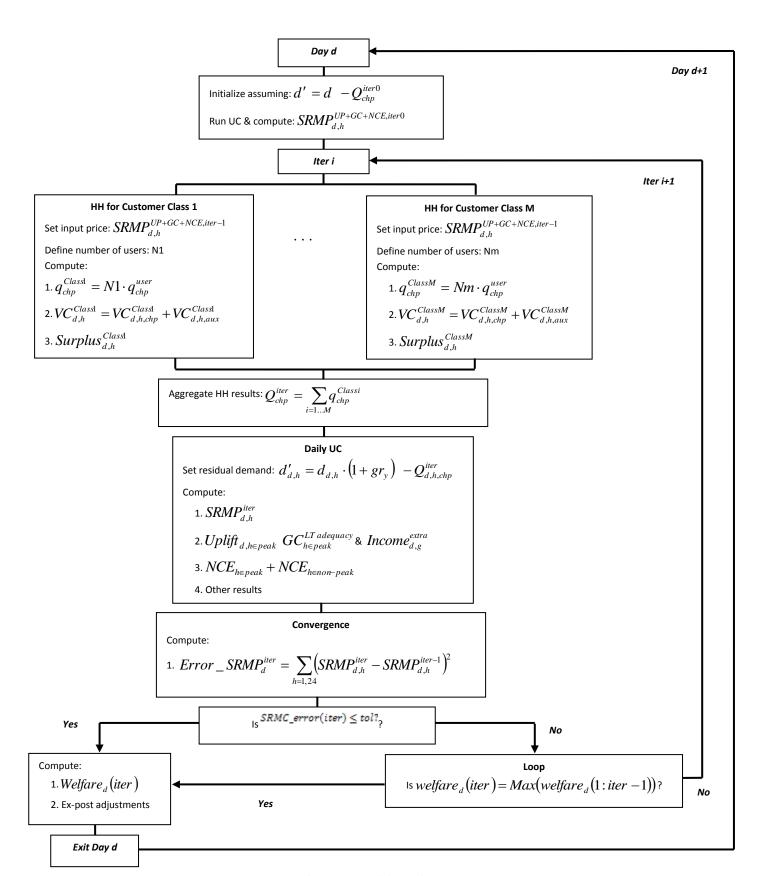
Figure 5.1.7: Short-term model complete iterative process
