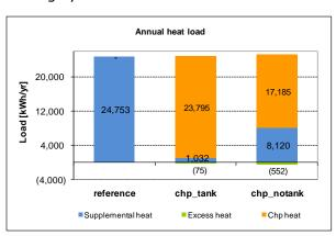
Figure 4.1.2b: Annual supplemental heat, micro-chp heat and excess heat
