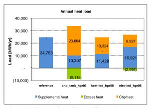
Figure 3.2.4b: Annual supplemental heat, micro-CHP heat and excess heat for low HPR
