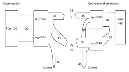
Fig. 1. Cogeneration versus conventional generation [4], where  $\alpha_E$ , part of the energy transformed into electricity in a cogeneration unit,  $\alpha_Q$ , part of the energy transformed into usable in a cogeneration unit,  $\eta_E$ , electrical yield of an electrical power plant (production of electricity only),  $\eta_Q$ , yield of a boiler (production of heat only), E, electricity demand, E, heat demand.
