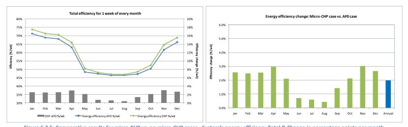
Figure 6.2.5: Comparative results for micro-CHP vs. no micro-CHP cases - System's energy efficiency Total & Change in percentage points per month
