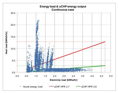
Figure 4.3.2: : Hourly electricity load vs. heat load
