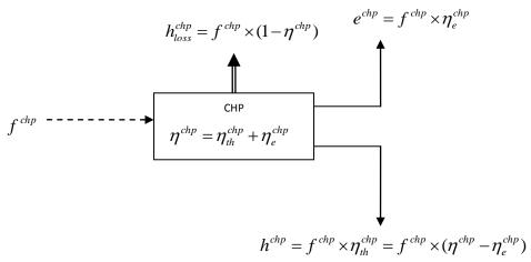
Figure A. 1 Micro-CHP energy outputs
