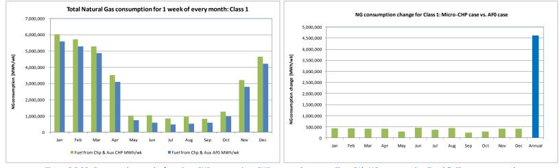
Figure 6.2.20: Comparative results for micro-CHP vs. no micro-CHP cases – Customer Class C1's NG consumption Total & Change per month
