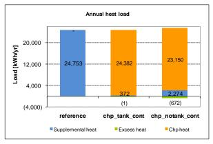
Figure 4.1.10b: Annual supplemental heat, micro-chp heat and excess heat for continuous case
