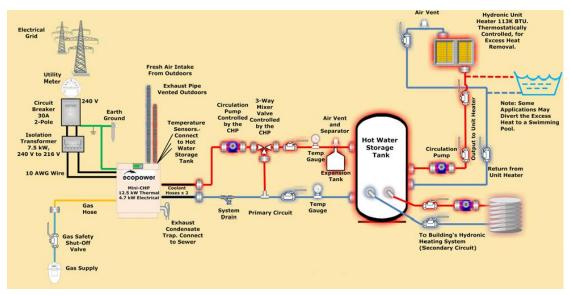
Figure 3. 1: Heating system with small-CHP
