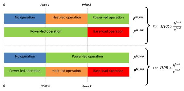
Figure 4.3.1: Micro-CHP operational outputs and conditions for Pse\_imp > Pse\_exp
