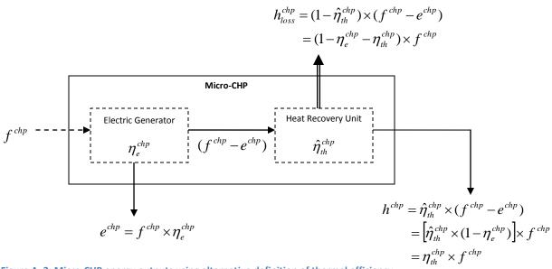
Figure A. 2: Micro-CHP energy outputs using alternative definition of thermal efficiency
