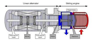
Figure 2.2.3: Free Piston Stirling Engine
