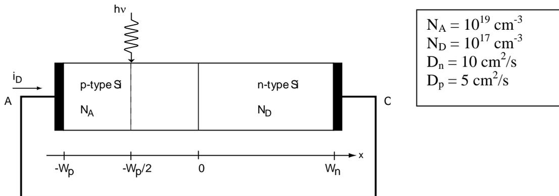
The p-n diode shown above is illuminated by light which generates  $G_L$  hole electron pairs per second in the plane at  $x = -W_p/2$ . This illumination results in an increased electron & hole population at  $x = -W_p/2$ . You are not given  $G_L$ , but you are told that  $n'_p(-W_p/2) = [n_p(-W_p/2) - n_{po}] = 10^{11} \text{ electrons/cm}^3$ .
