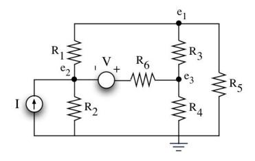
**3.** *[24 Points]*: Parts (A) through (C) of this problem analyze the network shown below by two methods: superposition and the direct application of the node method. You should compare for yourself the work required to analyze the network by these two methods. For Parts (A) through (C), assume that the port terminals to the right are left open.
