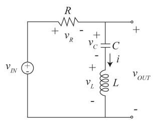
a) First, experimentally measure the step response of the network. To do so, log into iLab, and select the ELVIS Lab Client. When you launch the lab client, you will see the network on the canvas. Select the signal generator (FGEN) and set its parameters to WaveForm = SQUARE, Frequency = 1 kHz, Amplitude = 1 V, and Offset = 0 V. Next, select the output measurement unit (SCOPE) and determine a suitable
