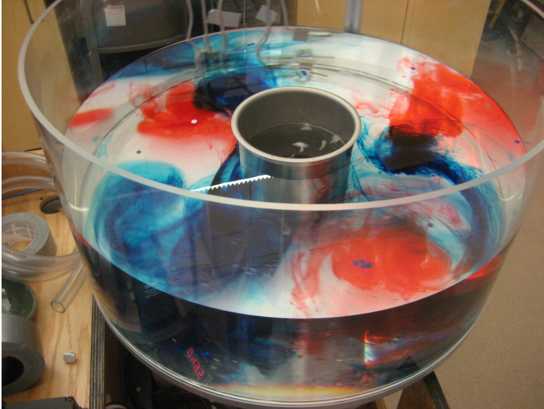
Figure 18: Turbulent Eddies in the High-Rotation Rate Tank Experiment. Some eddies are moving cyclonically about a low (counterclockwise) while others are moving anticyclonically about a high (clockwise). There is vertical 'stiffness' to these eddies; they do not vary vertically, only horizontally, as predicted by the Taylor-Proudman Theory.
