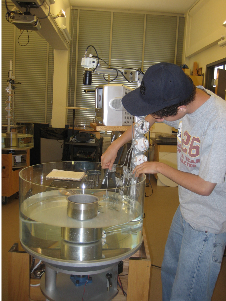
Figure 4: Experiment Setup. Vince examines the temperature sensors on the tank. Temperature sensors are along one 'longitude' so that we can examine one \partial T/\partial r and examine thermal wind balance in that region; we assume that the tank will have azimuthal symmetry and that jets and temperature gradients will be the same at each radius, regardless of 'longitude'.
