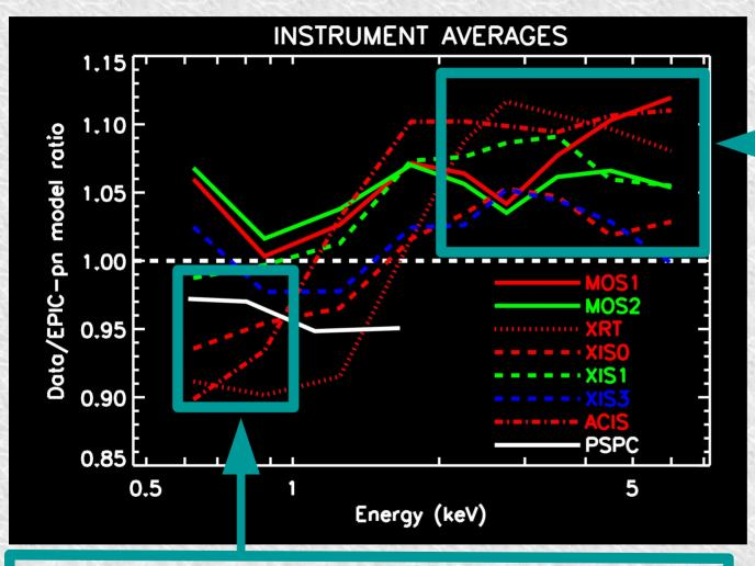
Most instruments show lower flux than pn at < 1 keV, but with a varying degree (0-10%)
