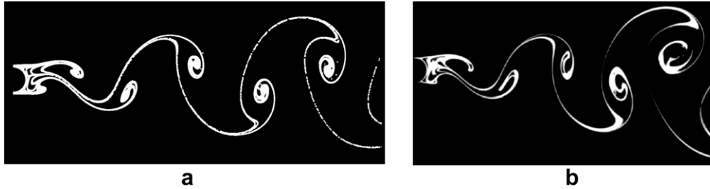
Fig. 4. Validation for (a) numerically resolved streaklines for Re = 100 (b) experimental visual of Taneda [38] for Re = 140 . Note in particular, the remarkable similarity in the eddy shedding process and the connection between all the shed eddies through an umbilical chord .
