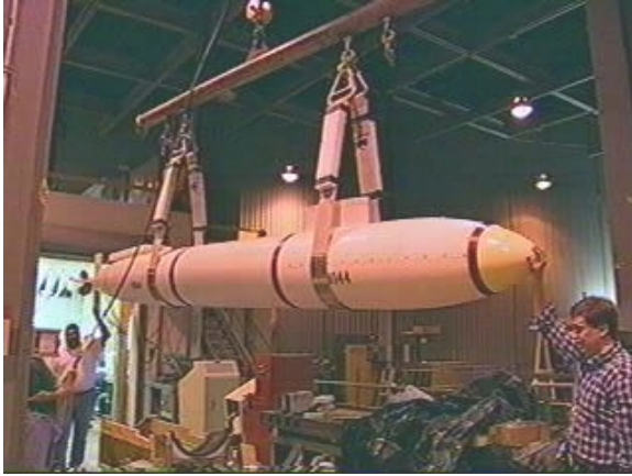
Fig. 6 NSWC 1/20-Scale radio-controlled free-running submarine model
