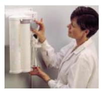
As long as the green LED is on, the water quality is above 1 M $\Omega$ .cm at 25 °C. When the LED is red, it's time to change the purification pack (DI-PAK®).
