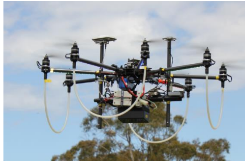
Figure 56 – Experimental Multirotor-copter Equipped with LiDAR
