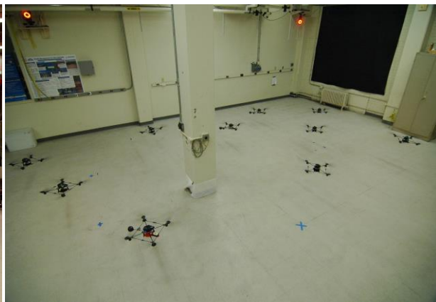
10 UAV quadrotors flying autonomously. The team flight is initiated by a single operator. (March 2007) - Courtesy Professor. Jonathan How, MIT
