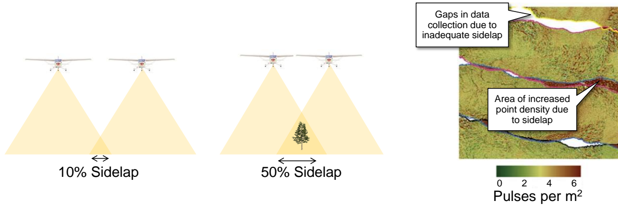
Figure 68 – Illustration of Sidlap and Impact on Data Collection
