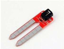
Two wire resistive sensor - excludes microcontroller - equivalent to home made solution ~$10
