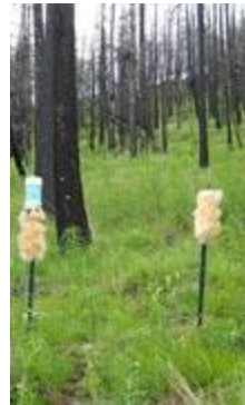
Autonomous recording unit (ARU,) developed by Cornell University to remotely count bird species
