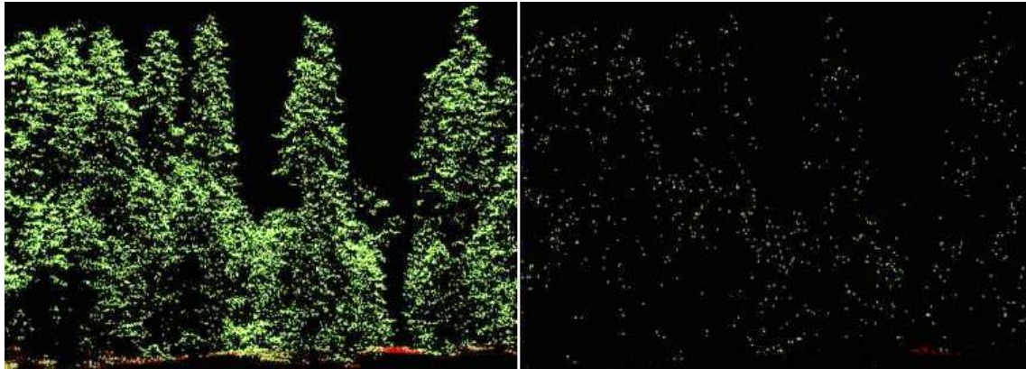
Figure 66 – Example Side Profile of Forest LiDAR Data: 8 pulses per m 2 vs. 0.25 pulses per m 2
