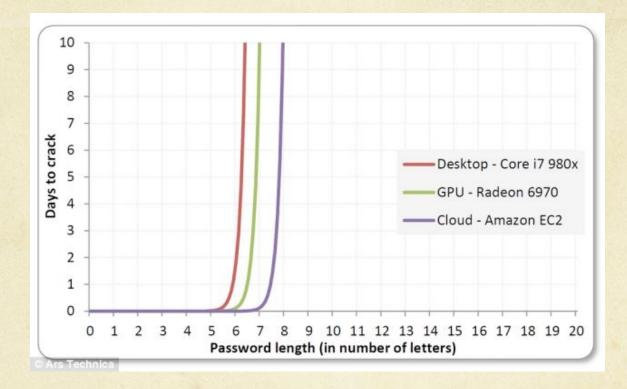
This graph shows how long in days it took the Ars Technica hackers to crack the list of 16,449 hashed passwords based on the method used. It also shows how long it took to crack passwords based on how long they were. Each hacker used a combination of wordlists, brute-force attacks and Markov chains to crack the list. One hacker managed to crack 90% of the list.
