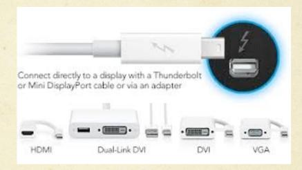
Exploit code can be passed through the Option ROM of any TB Adapter to a Mac which (now infected) can then pass the infection on to the Option ROM in another TB adapter.
