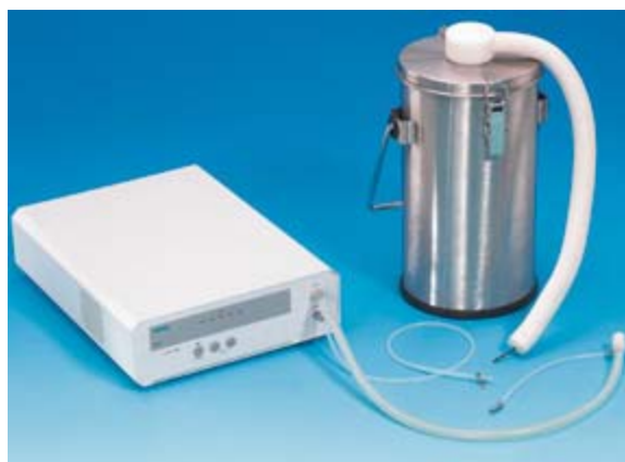
Figure 5: Liquid Nitrogen Pump (LNP94) and Dewar Flask
