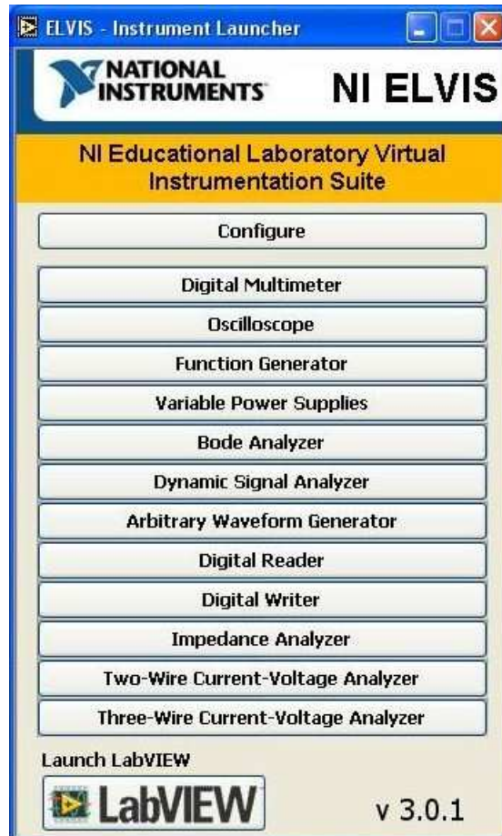
Figure 3-1: NI ELVIS software suite. Users can control the different instruments from this user friendly panel.
