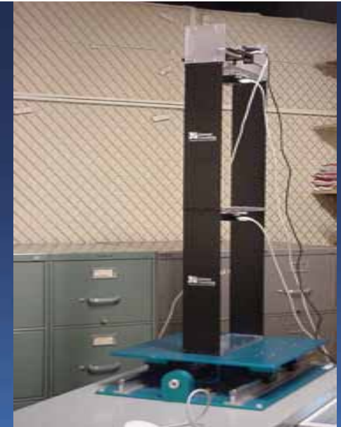
Shake table (Civil Eng., deployed 2004)
