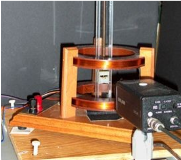
Figure 1. Force on a Dipole experiment located at MIT
