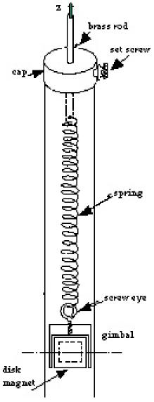
In this lab we will have a disk magnet (a dipole) suspended on a spring, which we will use to observe force s on dipoles due to different magnetic field configurations.
