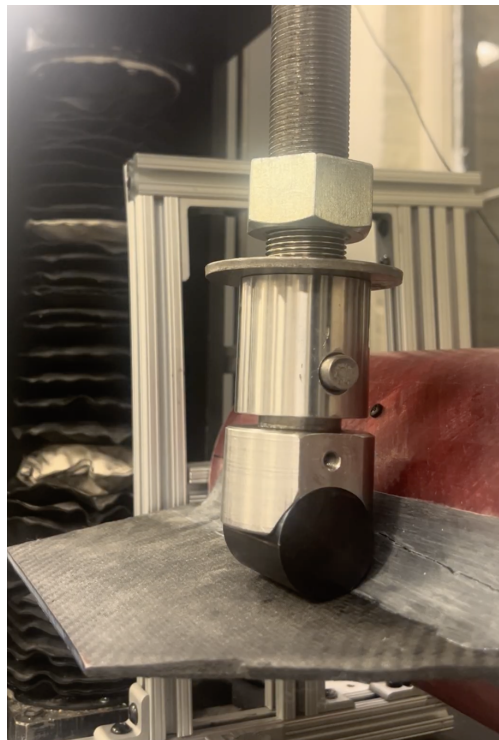
Figure 3: Close-up of the rounded compression fixture contacting the loaded carbon fiber fin near the end of the epoxy fillet.
